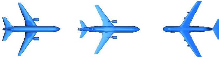
Figure 2.10: Three airplane models after pose normalization: major axes are correctly found but the front of the fuselage of the rightmost model is in the opposite direction.
